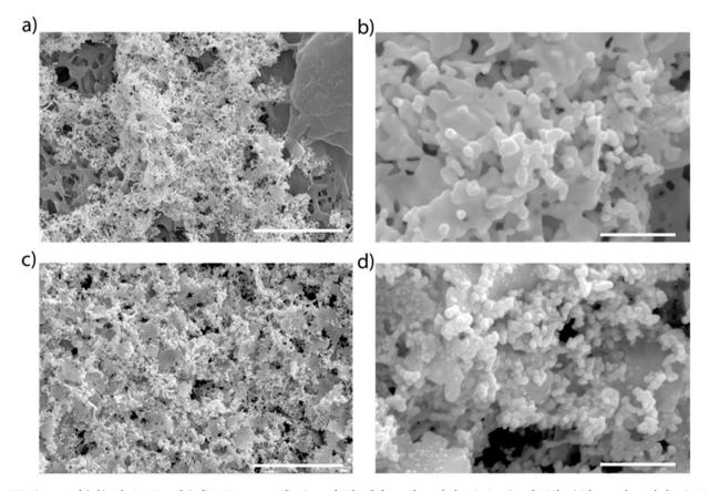
Fig. 2. SEM images of (a,b) 6 h AuNFs and (c,d) RNFs at magnifications of 20kx (left panels, scale bar is 4  $\mu$ m) and 100kx (right panels, scale bar is 500 nm). Following chemical roughening, the emergence of high density, ~20–50 nm nanoscale features is apparent.
