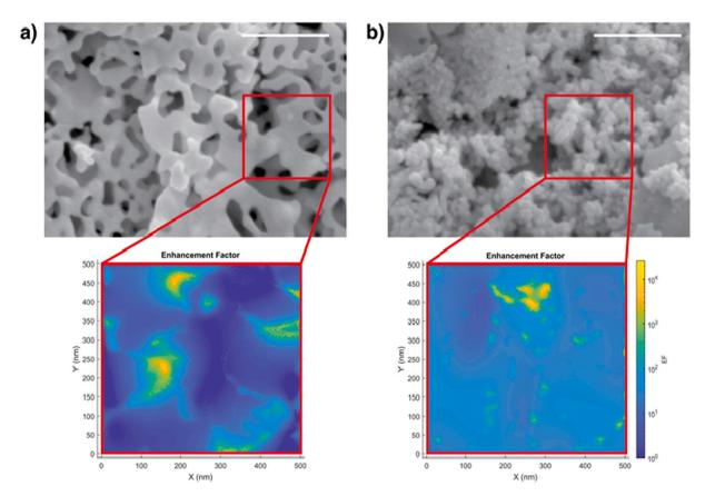
**Fig. 4.** FTDT simulation of electromagnetic enhancement. Topological features extracted from SEM images of AuNFs (a) and RNFs (b) were used to model the local EF of the substrates. RNFs feature a homogeneously increased EF throughout the substrate (insets represent roughly the optical focal area during scanning). Scale bar = 500 nm.
