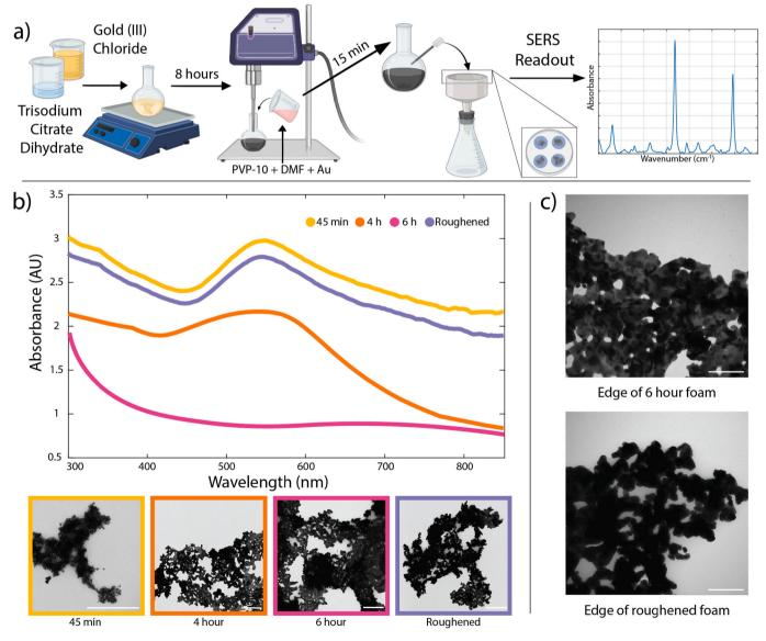
**Fig. 1.** a) Overview of hierarchically tuned nanofoam synthesis and deposition onto filter paper. b) UV–vis spectra and corresponding TEM images of nanofoams at time points 45 min, 4 h, 6 h, and after chemical roughening. Scale bar is 500 nm for all images. c) TEM images of the edges of normal foams at the 6 h timepoint (top) and roughened nanofoams (bottom), scale bar 100 nm.
