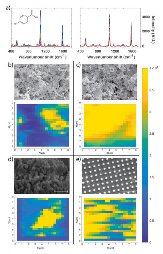
Fig. 3. Raman scanning of various SERS substrates with 4-MBA. Each raster scan represents an 8  $\mu$ m by 8  $\mu$ m area with a step size of 400 nm. a) Representative spectra of 4-MBA for AuNFs (left) and RNFs (right). SEM image and raster scan intensity at 1077 cm<sup>-1</sup> for b) AuNFs, c) chemically roughened RNFs, and commercial d) Ocean Optics and e) Hamamatsu SERS substrates. All scale bars are 1  $\mu$ m.
