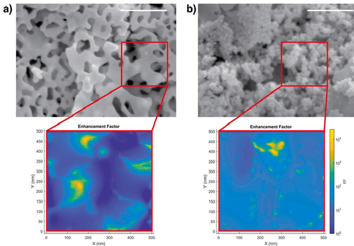
**Fig. 4.** FDTD simulation of electromagnetic enhancement. Topological features extracted from SEM images of AuNFs (a) and RNFs (b) were used to model the local EF of the substrates. RNFs feature a homogeneously increased EF throughout the substrate (insets represent roughly the optical focal area during scanning). Scale bar = 500 nm.
