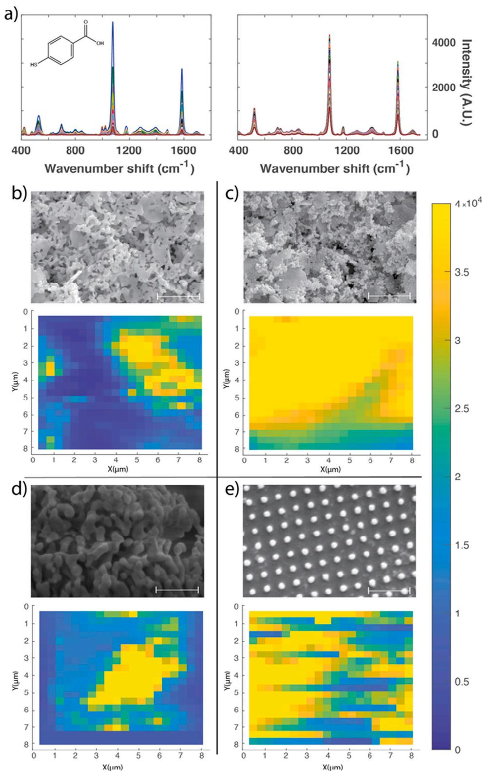
**Fig. 3.** Raman scanning of various SERS substrates with 4-MBA. Each raster scan represents an  $8 \mu\text{m}$  by  $8 \mu\text{m}$  area with a step size of  $400 \text{ nm}$ . a) Representative spectra of 4-MBA for AuNFs (left) and RNFs (right). SEM image and raster scan intensity at  $1077 \text{ cm}^{-1}$  for b) AuNFs, c) chemically roughened RNFs, and commercial d) Ocean Optics and e) Hamamatsu SERS substrates. All scale bars are  $1 \mu\text{m}$ .
