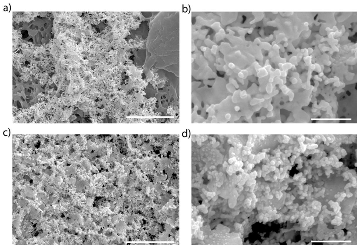
Fig. 2. SEM images of (a,b) 6 h AuNFs and (c,d) RNFs at magnifications of 20kx (left panels, scale bar is 4  $\mu\text{m}$ ) and 100kx (right panels, scale bar is 500 nm). Following chemical roughening, the emergence of high density, ~20–50 nm nanoscale features is apparent.
