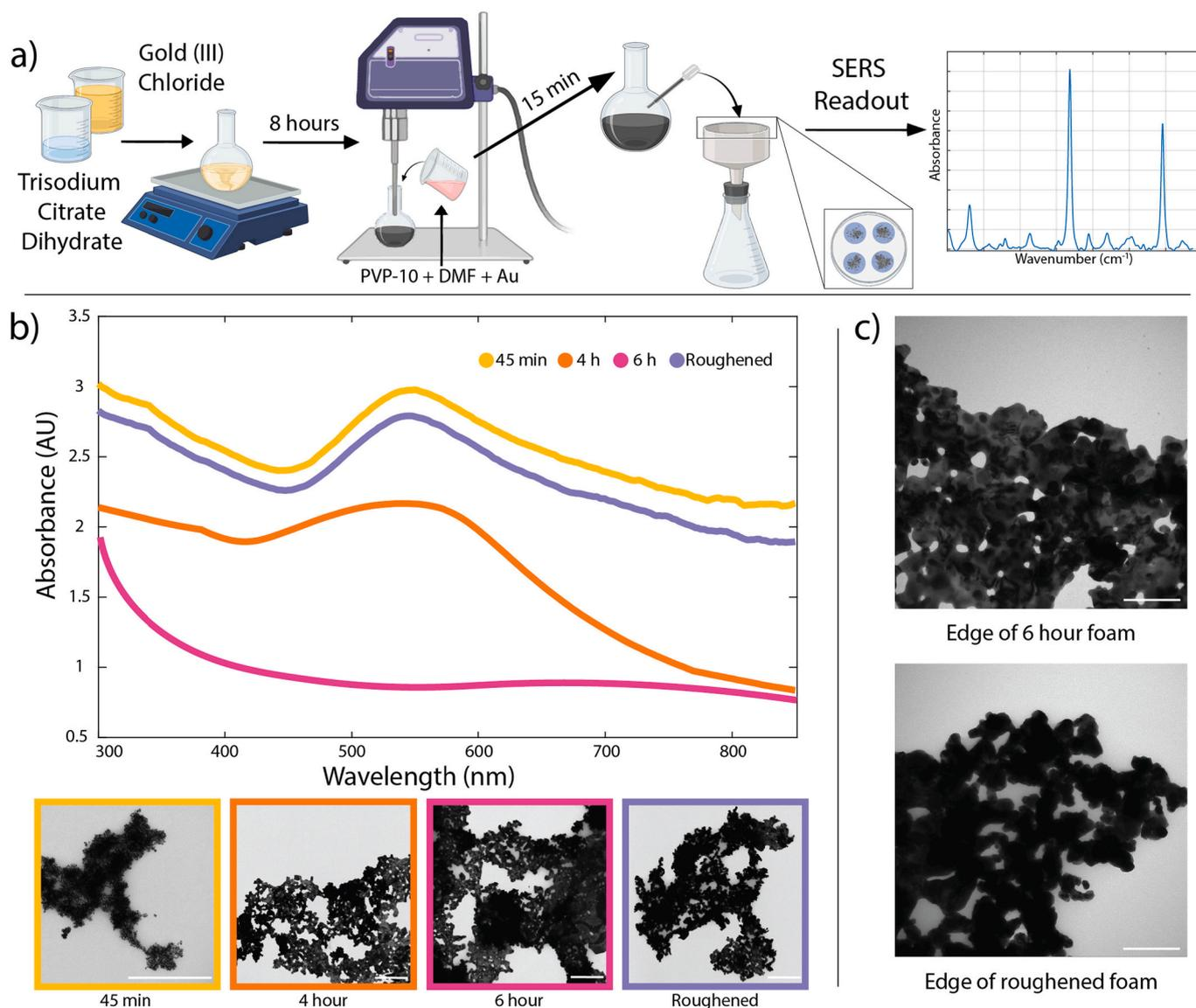
**Fig. 1.** a) Overview of hierarchically tuned nanofoam synthesis and deposition onto filter paper. b) UV-vis spectra and corresponding TEM images of nanofoams at time points 45 min, 4 h, 6 h, and after chemical roughening. Scale bar is 500 nm for all images. c) TEM images of the edges of normal foams at the 6 h timepoint (top) and roughened nanofoams (bottom), scale bar 100 nm.
